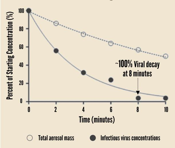
Data from test at 20% relative humidity and 100% light intensity
